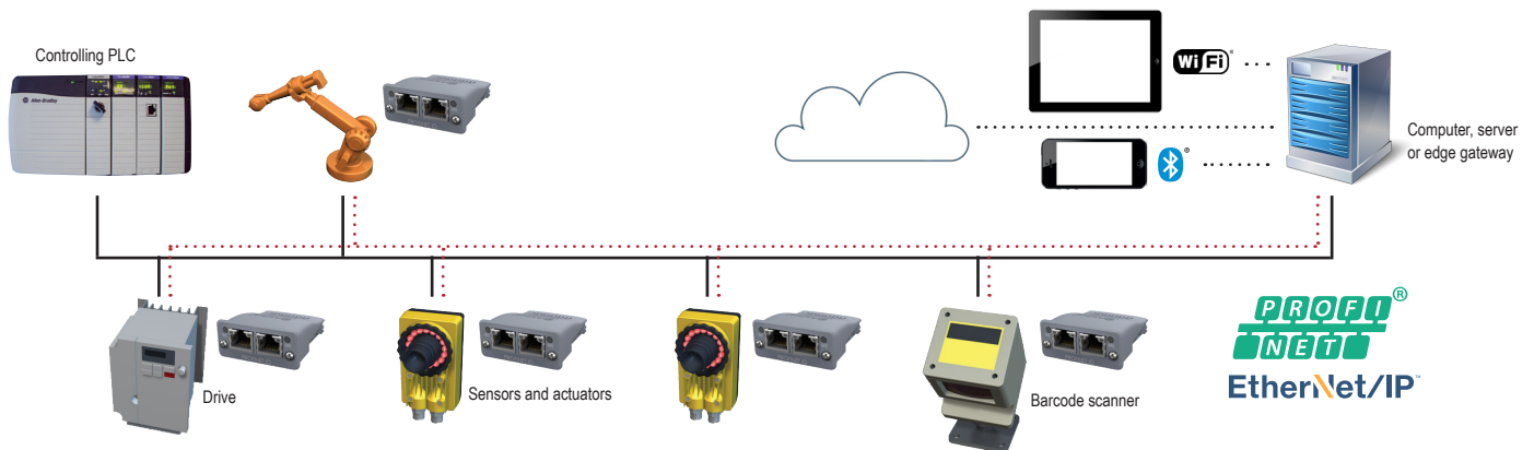
Example use case of an industrial network using the Anybus CompactCom OPC UA or MQTT functionality.
